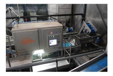
The Focus is an optical sorter, especially developed to sort products with various optical deficiencies. At the product flow discoloration, deformation and foreign objects are detected and removed accurately. The Focus can be used for fresh/dried or frozen crustaceans and shellfish, like mussels, cockles and shrimps. Use of the Focus will lead to quality improvement of your final product, but also to a stable quality, resulting in lower production costs.
