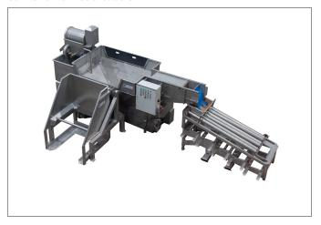
The principle of the universal sorter is based on revolving rollers, which consist of sets of 2: one roll is provided with a spiral, the other one is a smooth one and together they take care of the transport of the product, one by one. All rollers are individually driven by a drum motor.
