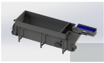
Cooling water is applied to the product via sprinkler irrigation. This allows us to use the most optimal cold transfer. The tires are equipped with a spray system in the frame to automatically clean them from the inside.
