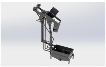
An additional advantage is that the stone remover also has a washing effect on the product. Several choices are possible for the circulation flow of the water.
