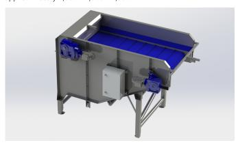
This machine is equipped with a vertically movable conveyor belt with carriers; the belt moves up and down with the product flow. This has the advantage that the drop height is minimal, and the product cannot be damaged by fall.
