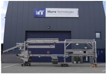
The drives are with drum and slip-on motors and the bearings are heavy duty, with bearing housings filled with grease that is foodsafe.
