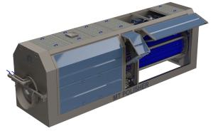
A heavy-duty belt has been chosen for rotating the drum. Hereby, the drum is supported by idlers. The brush rollers rotate via v-belts and are fitted with ball bearings. Our design also ensures that there is a maximum distance between the brush rollers of 3 mm, resulting in minimal
