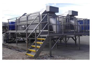
The drum hangs in 2 heavy-duty toothed belts that together have one drive and the shafts are equipped with heavy duty food safe grease-filled bearing housings. Process water is collected under the machine in a water tank.
