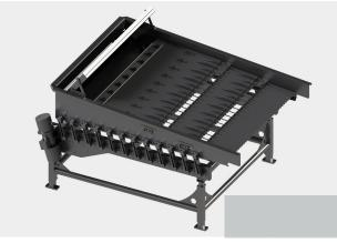
The machine is indirectly driven by 2 unbalance motors and features an infeed section to effectively spread the product across the entire width of the sorting table. The carrots are then positioned longitudinally by means of aligning plates with V-tracks. Two infinitely adjustable openings are fitted in the longitudinal direction to sort out on 2 different bottom sizes.
