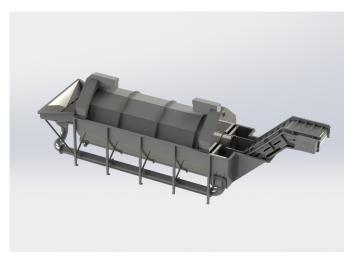
The drum hangs in 2 heavily toothed belts that each have their own drive system. Because the pumping system is mounted directly on the back of the water tank, washing can be done with minimal energy consumption because the water circulates from the inlet to the outlet.
